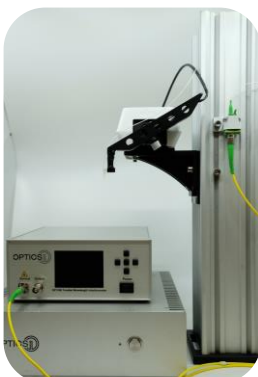
7. Doublecheck the fiber connections before starting the system
