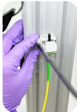
2. Mount the adapter & patch-cord to the sliding piece with the M6 screw
