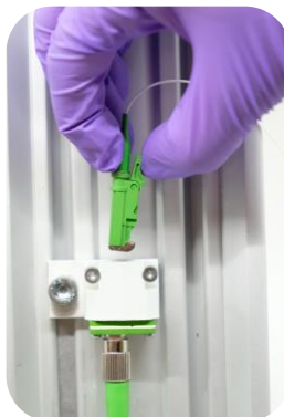
8. To disconnect the probe again, gently push the green lever of the new probe connector
