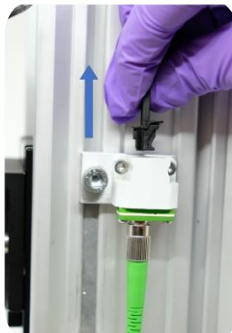
5. Remove the black cap from the adapter
