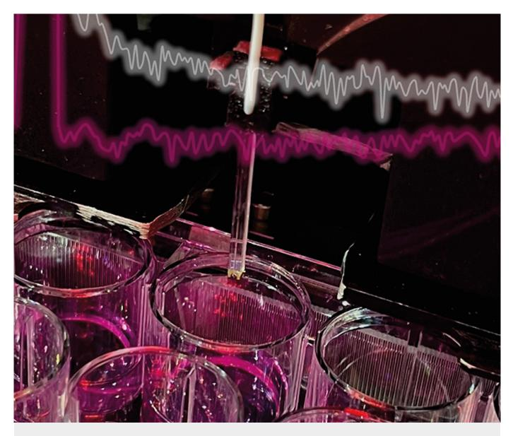
Next-generation dynamic cell stiffness measurements on the Pavone platform using multisine broadband excitation (spectral response illustrated).
