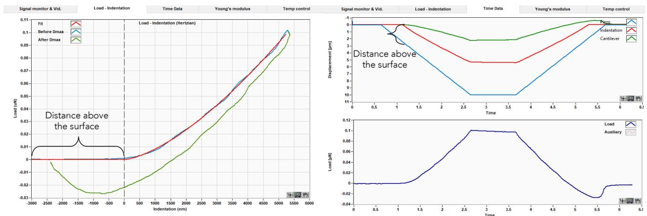
Figure 4: A correct load-displacement curve (left) and time data tab (right) after performing one indentation in D-mode from a certain distance above the sample surface.
