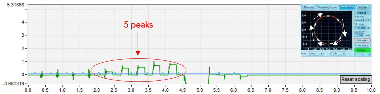
Figure 8: Live monitor signal: Find surface stops too late, already within the sample, indicated by five peaks (instead of one).
