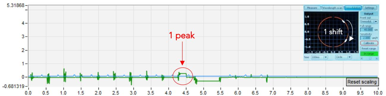
Figure 3: Live monitor signal in software: cantilever bending shown as green baseline, Piezo extension as blue line
