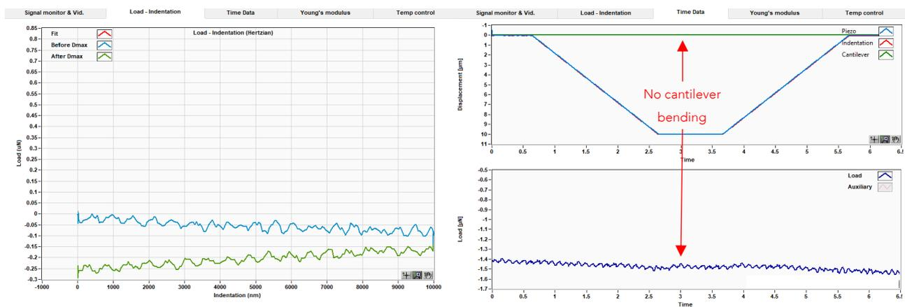
Figure 7: Load-displacement curve (left) and time data tab (right) after performing one indentation in D-mode, showing no cantilever bending, hence no surface detection.
