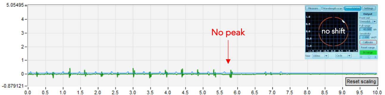
Figure 6: Live monitor signal: Find surface stops too early, close to the sample surface.
