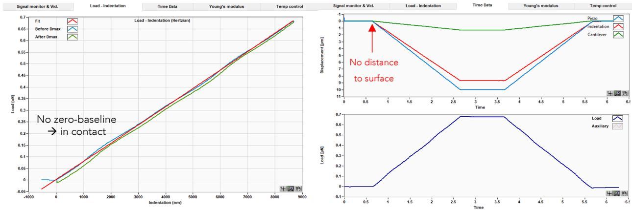
Figure 9: No Zero-baseline in Load-displacement curve (left) and no distance to surface shown time data tab (right), indicating that the measurement was performed when the probe was already in contact with the sample surface.
