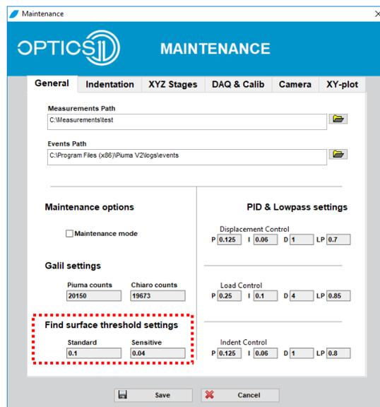
Figure 2: Maintenance menu with Find surface threshold settings
