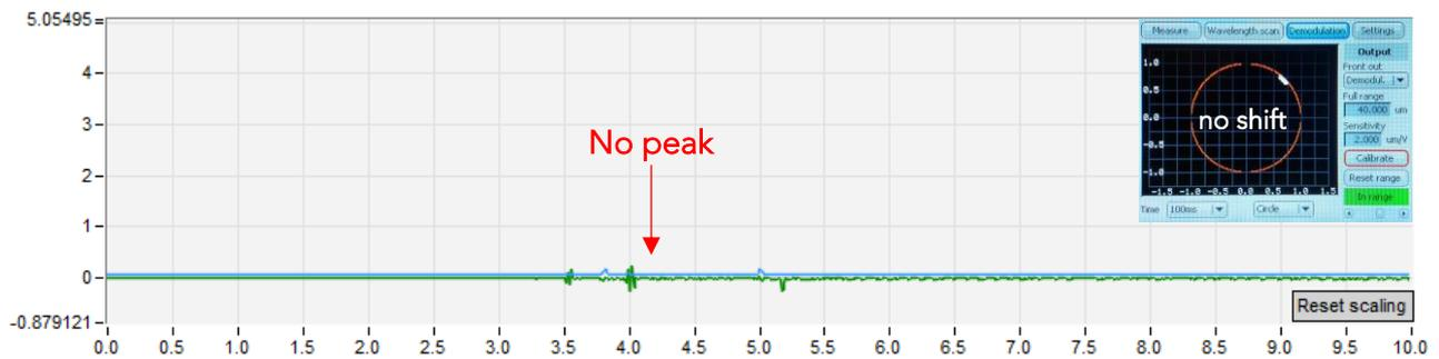
Figure 5: Live monitor signal: Find surface stops too early after initial steps.
